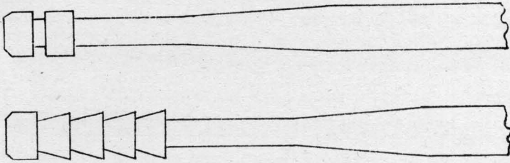
Figure 7. Proper design of tips for rifle rod
